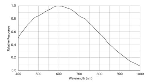
The spectral response curve excludes lens characteristics and light source characteristics.
