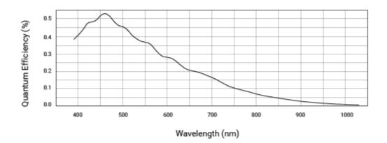
The spectral response curve excludes lens characteristics and light source characteristics.
