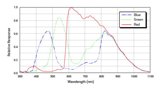
The spectral response curve excludes lens characteristics, light source characteristics, and IR cut filter characteristics.
