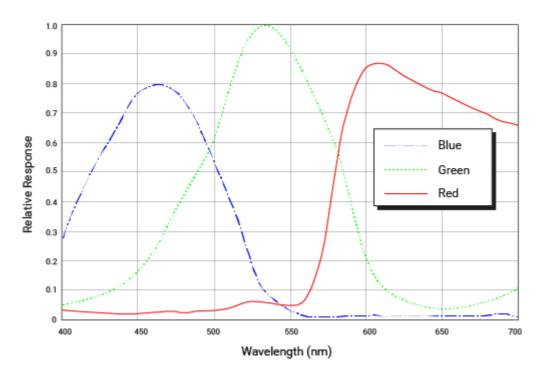
The spectral response curve excludes lens characteristics, light source characteristics, and IR cut filter characteristics.
