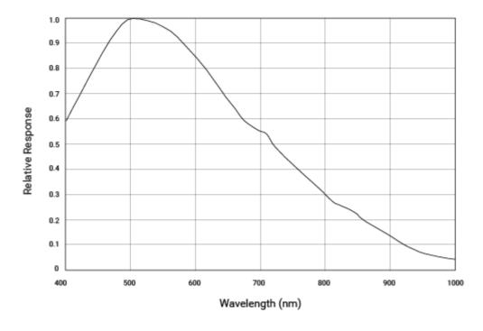
The spectral response curve excludes lens characteristics and light source characteristics.
